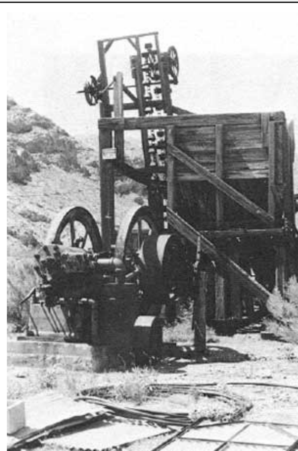
Illustration 71. Hot-shot diesel engine and ore bin, Gold Hill Mill site. Photo by Linda W. Greene, 1978.
